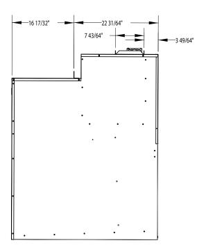
NOTE: Unit must be mounted a minimum of 8 inches above finished floor. See installation guide for vent termination clearances
