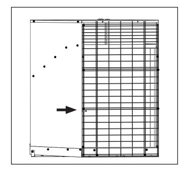
8. Alternatively, if the model does not have a 3/8" hole on the right side of the coil run the white temperature sensor over the fan deck and hang on the outside of the grille. Use the entire length of the wire getting the sensor as far down the back side of the unit as possible. On the fan deck use foil tape to secure the wire.
