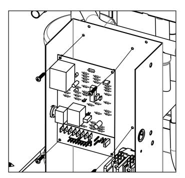
3. Align the defrost board bracket with the four holes in the control box and secure it using the four sheet metal screws.
