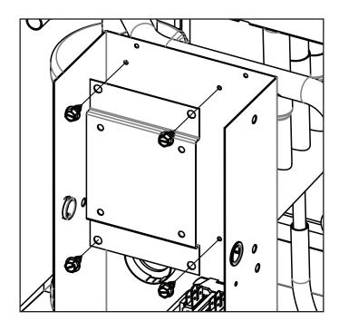
4. Carefully insert the four plastic standoffs to the new control board.
