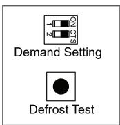
If using **ALTERNATIVE POSITION** of the ambient temperature sensor select **DEFROST CURVE 1** for the dip switch settings.
