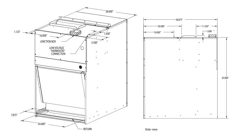
NOTE: Unit must be mounted a minimum of 8 inches above finished floor.
