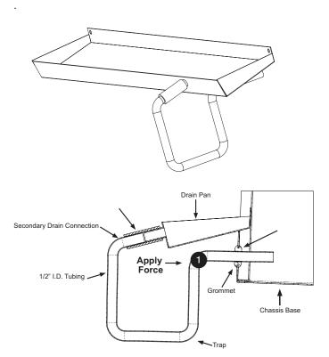
**4.** Position the trap as shown and slide the 2" piece of clear flexible tubing about 1" onto the top end of the trap. Slide the top of the flexible tube on the trap onto the bottom of the 1/2" OD secondary drain connection and push the top of the trap up. The trap should be positioned so that there is only a small gap between the top of the trap and the bottom of the secondary drain connection.
