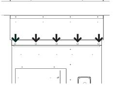
NOTE: FOR EASE OF INSTALLATION, INSTALL THE CABINET INTO THE WALL SLEEVE FIRST WITHOUT THE COOLING CHASSIS. THEN SLIDE COOLING CHASSIS IN AFTER CABINET IS IN PLACE.
