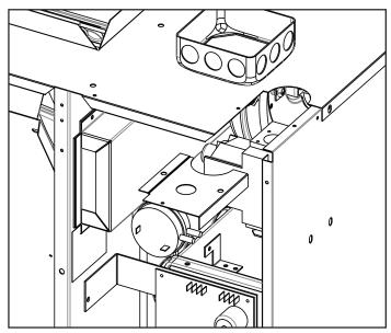
**3.** Remove (2) right side screws and remove the front furnace baffle.
