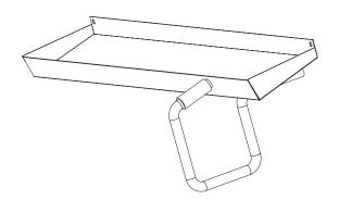
**4.** Position the trap as shown and slide the 2" piece of clear flexible tubing about 1" onto the top end of the trap. Slide the top of the flexible tube on the trap onto the bottom of the 1/2" OD secondary drain connection and push the top of the trap up.
