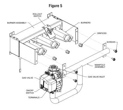
NOTE: IF ANY OF THE BURNER COMPONENTS ARE DAMAGED OR DETERIORATED, REPLACE THE BURNER ASSEMBLY.
