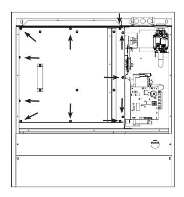
4. Remove front furnace baffle.
