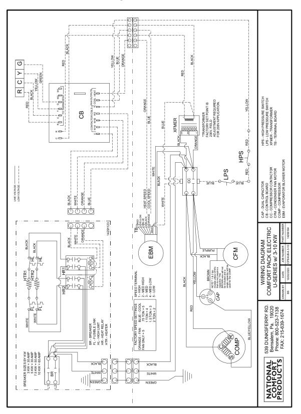
Wiring Schematic - 3-10kW
