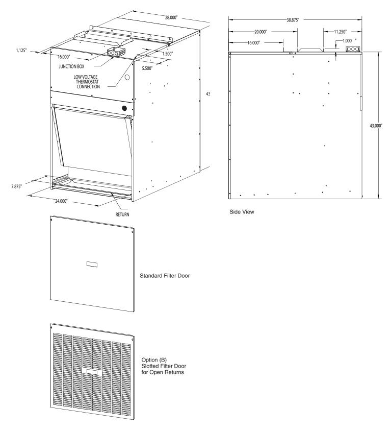
NOTE: Unit must be mounted a minimum of 8 inches above finished floor.
