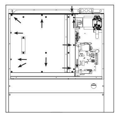
**7.** Remove front furnace baffle.
