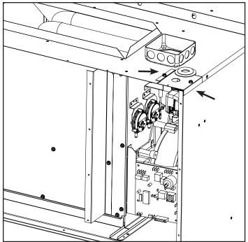
2. Remove the top heater mounting bracket of freeze protection.
