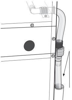
Clear tubing to fit into field installed drain line. There must be an air gap surrounding the clear tubing
