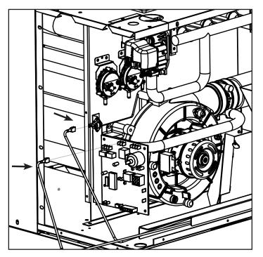
3. Slide out the freeze protection bracket.
